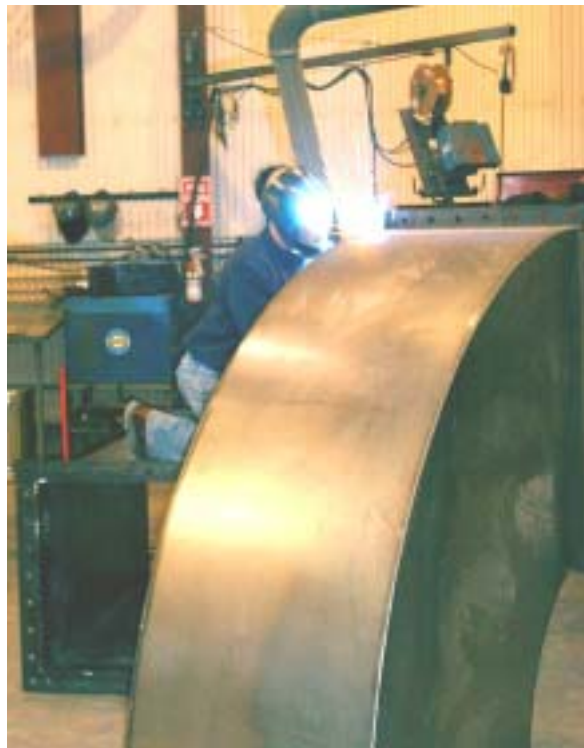
Brad Arkland is shown welding on the boiler breeching duct for Harvest States Oilseed Processing facility.
