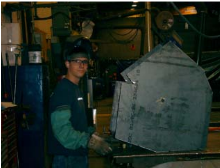
Shane Warner assembling a 16" square bucket valve for PMI-NE LLC
