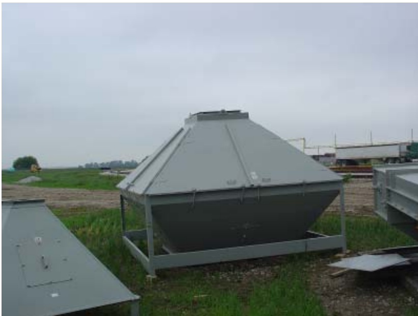
The scalper that crews will be installing at Aurora Coop.
